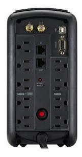
There should also be a USB cable connected from the USB port (white, top-right above) on the UPS, to a USB port on your computer. This is used to monitor the UPS from the **Power Panel Personal Edition** application on your FAST machine.
